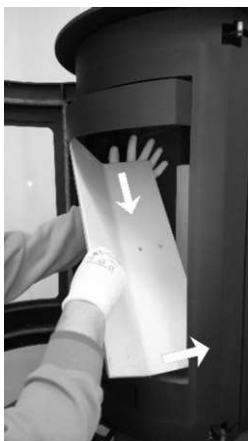
7. Push the metal deflector upwards. Grip the side concrete plate by the lower edge towards the centre of the fireplace. Pull it out through the door opening diagonally. Both sides evenly.
